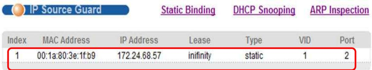
The screenshot shows the ZyXEL web interface for IP Source Guard configuration. The 'Static Binding' tab is selected. A table lists the configured entries:
